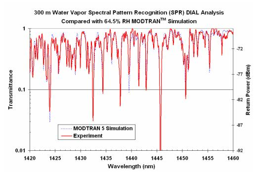
Fig. 9. Spectral measurement in the 1420 to 1460 nm infrared region with strong water vapor absorption features.
