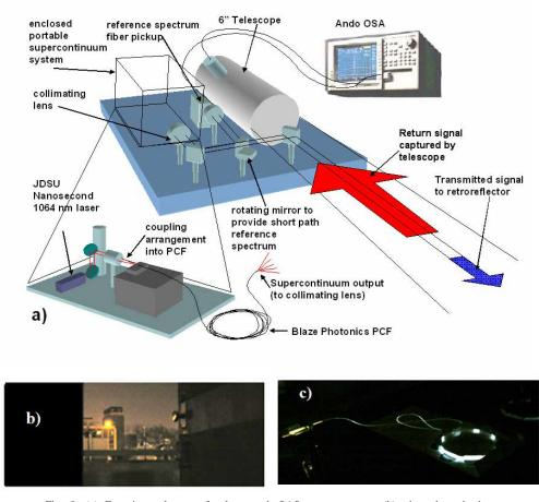
Fig. 8. (a) Experimental setup for long path SAS measurements; (b) view through the laboratory door shows the reflection of UV-NIR supercontinuum source from a 6" retroreflector located ~150 m away; (c) the wavelength spread of the supercontinuum light can be observed in the PCF, when it is properly tuned for maximum output power, it is spread in wavelengths through visible and near IR due to self phase modulation.
