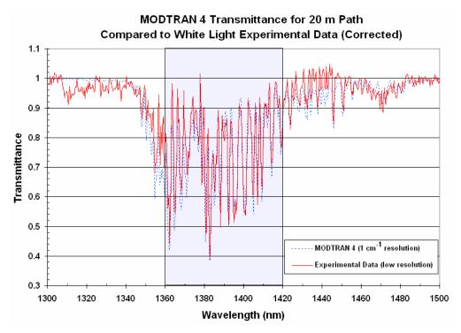
Fig. 3. Normalized water vapor transmittance 1300-1500 nm measurements using the supercontinuum laser (red) are compared when the spectrometer slit is set for the 1 cm<sup>-1</sup> resolution corresponding with of MODTRAN<sup>TM</sup> 4 (blue).
