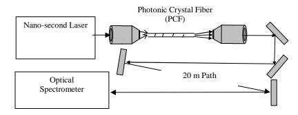
Fig. 2. Experimental setup used to measure water vapor spectrum with a supercontinuum source.
