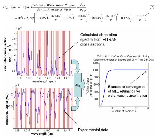
Fig. 6. Shown on the left is the calculated water vapor absorption spectrum (top) and experimental data (bottom). The red vertical lines are utilize a linearly spaced wavelength sampling scheme to feed spectral absorption information into the MLE algorithm. The algorithm iterates until it converges upon a best fit CPL (right), given the set of experimental data and absorption spectra of water vapor in a predetermined wavelength region.
