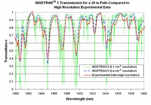
Fig. 5. Water vapor transmittance 1400-1420 nm experimental measurement (red) compared to MODTRAN<sup>TM</sup> 5 simulation with parameters selected to match the sensor (blue). The highest resolution available (0.1 cm<sup>-1</sup>) for MODTRAN<sup>TM</sup> 5 simulations (green) is also shown for reference.
