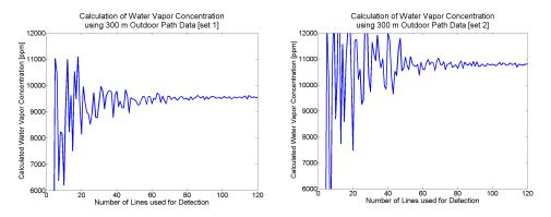
Fig. 10. Result of MLE algorithm for two 300 m path averaged measurements of water vapor.
