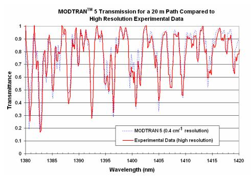
Fig. 4. Water vapor transmittance 1380-1420 nm experimental measurements (red) compared with MODTRAN<sup>TM</sup> 5 simulation (blue), with resolution matched to the instrument 0.4 cm<sup>-1</sup> parameter.
