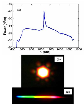
Fig. 1. (a) Supercontinuum source spectrum; (b) The far field pattern of the supercontinuum spectrum generated from a photonic crystal fiber; and (c) Rainbow observed after collimated light passes through a prism.
