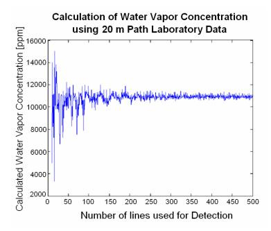
Fig. 7. Calculation of water vapor concentration showing the convergence using 10 to 500 laser lines for comparison.
